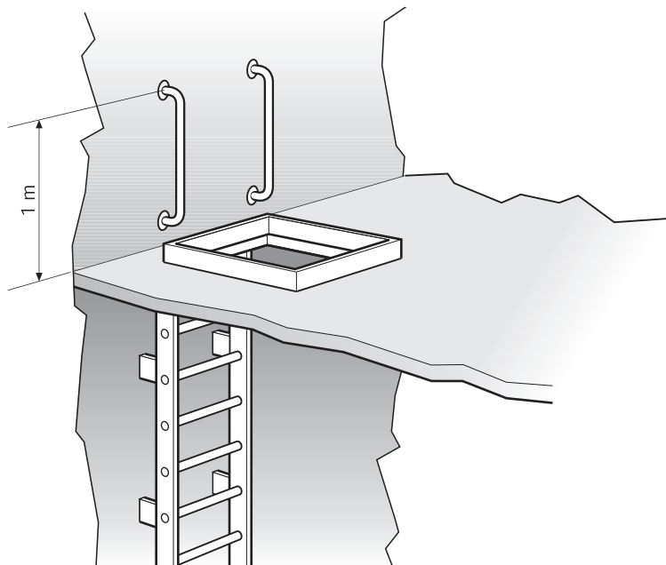
Figure 15. Vertical ladder through opening
