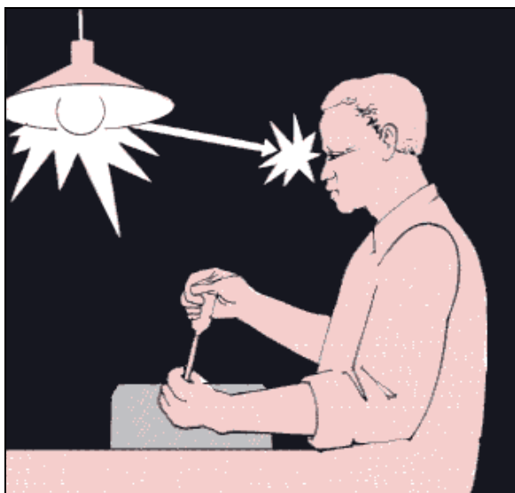
Glare from a low ceiling lamp, incorrectly positioned.
