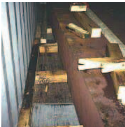
Figure 7.45 – Transverse blocking of steel slab
