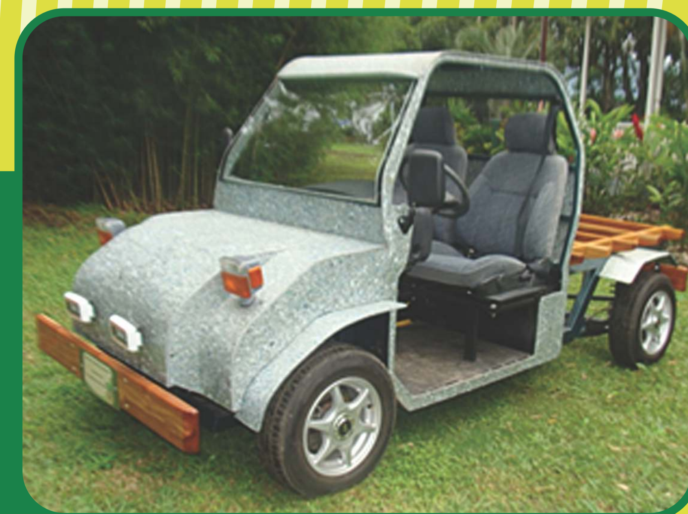
An electric vehicle prototype built at the Costa Rican National Training Institute with parts from other vehicles, the original design of the chassis, and the bodywork is constructed from tetra pack and other packaging waste collected from a dairy cooperative
