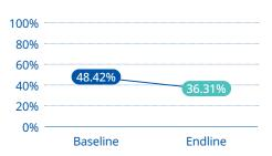
**Number of re-cuts:** Proportion of fabric used for re-cuts compared to the total amount of fabric used (corresponds to waste).
