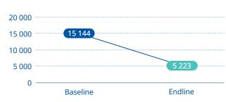
**Work in progress (WIP) level:** Amount of pieces not yet completed between two work stations. It is calculated separately for each line, or for all lines together (very low and very high WIP are signs that lines are not well balanced).
