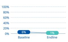
Finishing room defect rate (defects per 100 units): Average number of defects found per 100 inspected units (lower DHU indicates higher quality), can be calculated separately for each line, or for all lines together.
