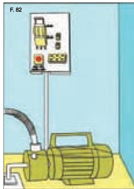
*Figure 82:* Clearly visible emergency controls of a pump attached to an electricity board.
