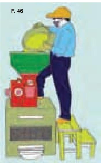
*Figure 46 : Adjust the work height by using a stable foot platform corresponding to your elbow level.*
