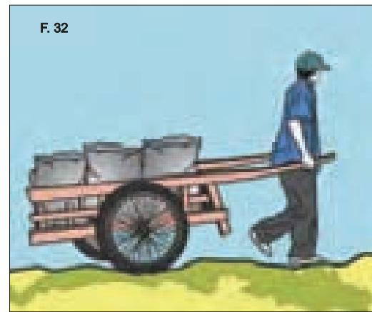
Figure 31, 32 : On rough roads, it is easier to push or pull hand-trucks with big wheels than those with small wheels.
