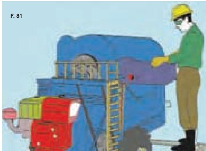
*Figure 81:* Place emergency control of the machine clearly visible and within easy reach of users..
