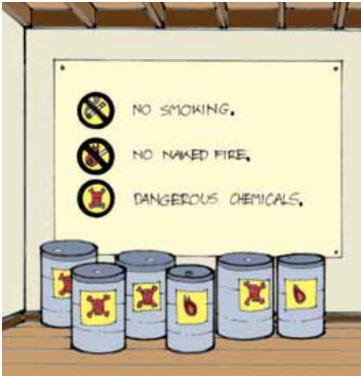
Figure 32: Store hazardous chemicals outside work areas with a firm lock. Ensure children do not come into contact with them.
