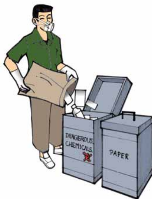
Figure 36: Collect waste bottles of dangerous chemicals in a separate container.
