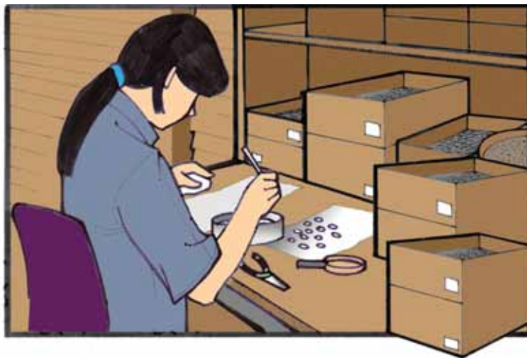
Figure 22: Use convenient materials containers to keep frequently-used materials within easy reach and in an orderly manner.
