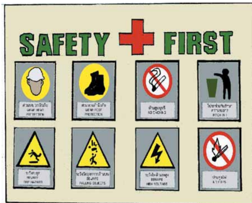
Figure 39: Alternatively consider using symbols to identify hazards – make sure everyone in the workplace knows what they mean!
