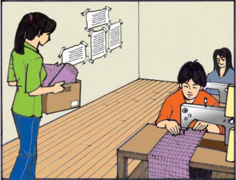
Figure 2: Clear passageway for smooth transportation of materials or products.
